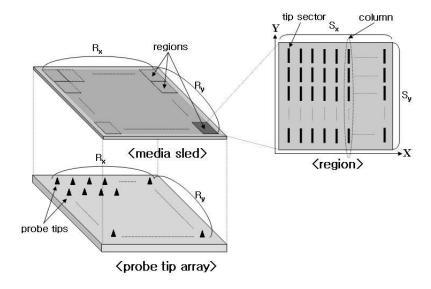
Figure 1. The structure of the MEMS storage device.
