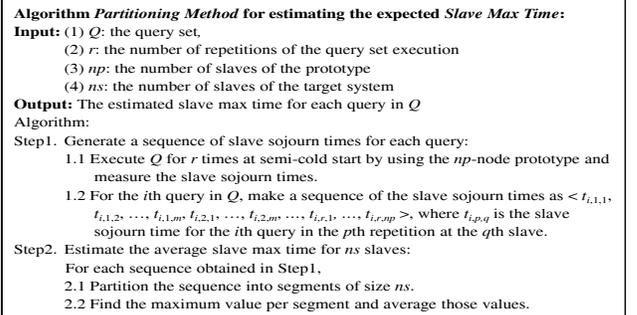
**Figure 9: The algorithm for estimating the expected slave max time by using the partitioning method.**
