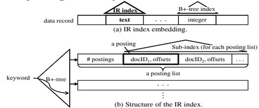
**Figure 3: The IR index of the DB-IR tightly integrated DBMS.**
