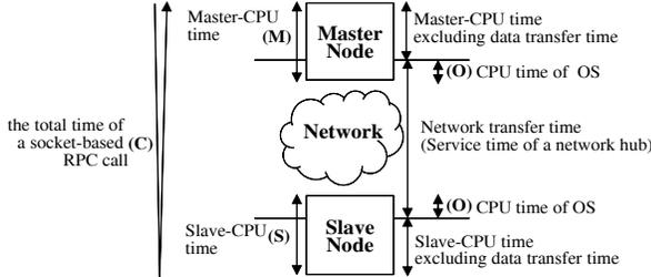
**Figure 8: Measurement of a service time at a network hub.**
