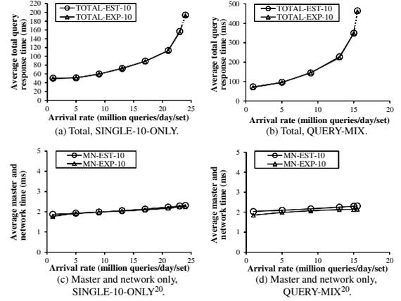
**Figure 11: The estimated and experimental results of the ten-node system ( $ns=10$ ) as the query arrival rate is varied. EST-10 represents estimated results for the 10-node system; EXP-10 experimental results.**
