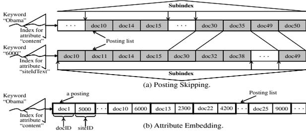
Figure 4: IR query processing in a tightly integrated DB-IR system [29].
