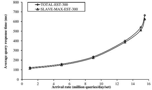
Figure 14: The projected average response time of ODYS for real-world scale service ( $ns=300$ ). TOTAL-EST-300 is the average estimated total query response time; SLAVE-MAX-EST-300 the average estimated slave max time.
